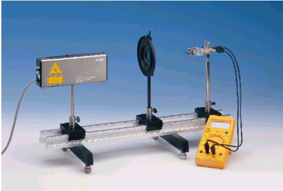
Figure 21: Experimental set-up: Malus' law [13]
